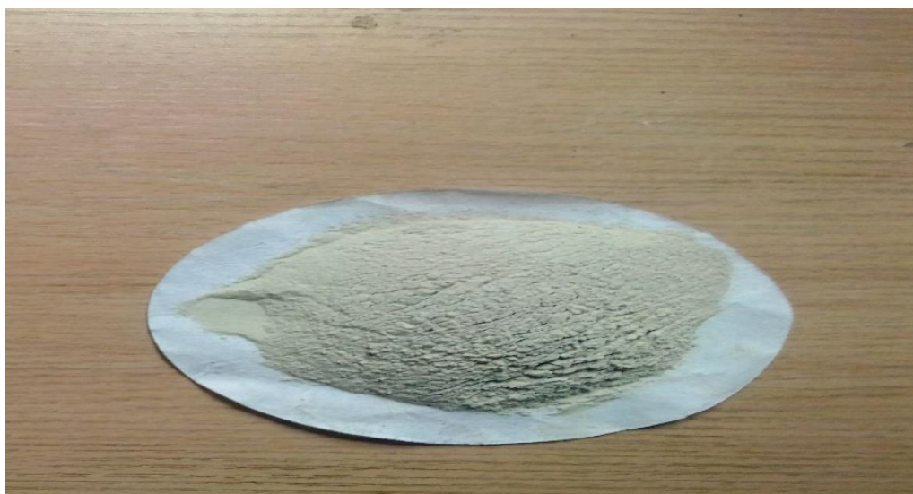
Fig. 3: A sample of Obubra baryte of size 75 \mu m obtained after milling
