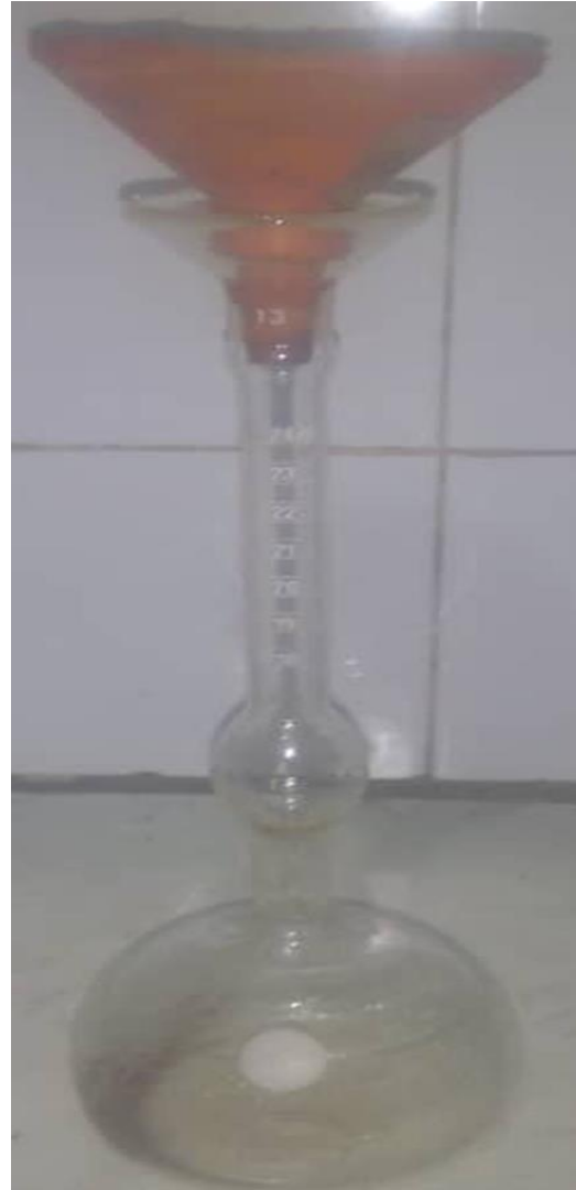
Fig 2b. Insertion of the funnel into the Le Chatelier flask
