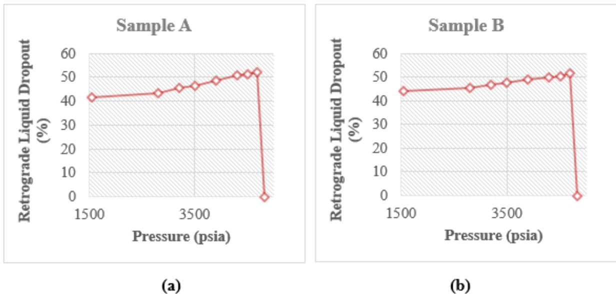
**Fig. 2:** CCE Retrograde liquid dropout plot for (a) sample A and (b) sample B
