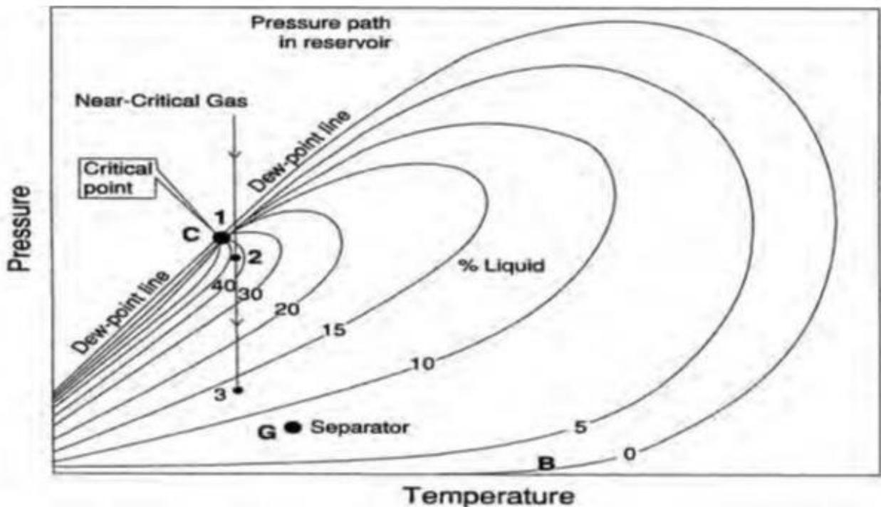
Fig. 1: Pressure-Temperature diagram of a near-critical gas condensate (Ahmed, 2006)
