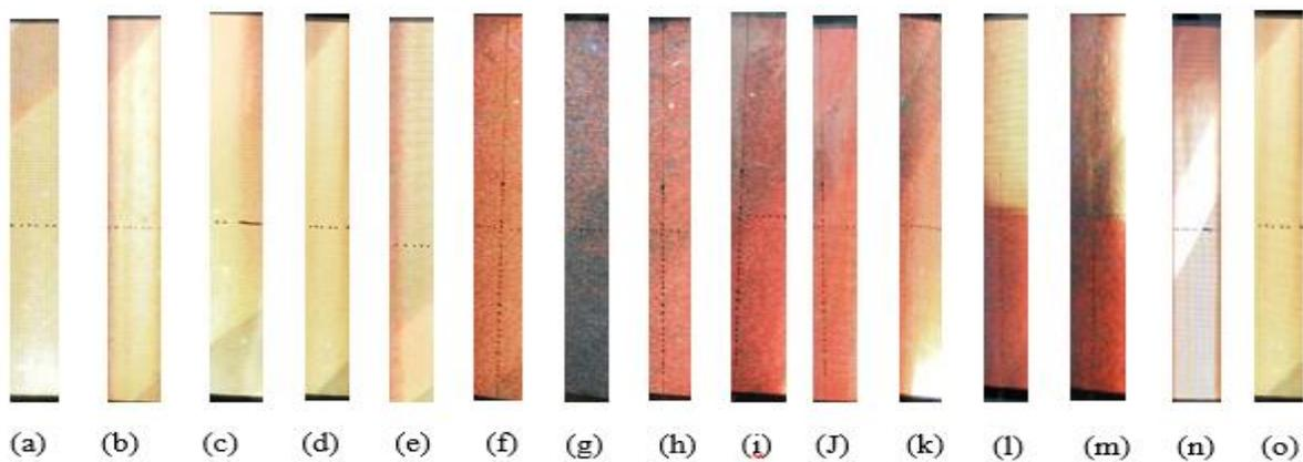
**Fig. 3:** Critical opalescence phase behaviour phenomena in the Constant Composition Expansion experiment at 101.7 °C
