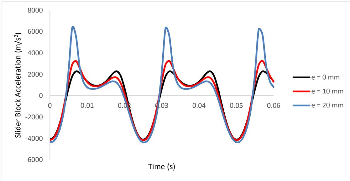
**Fig. 15:** Effect of offset distance on acceleration of slider
