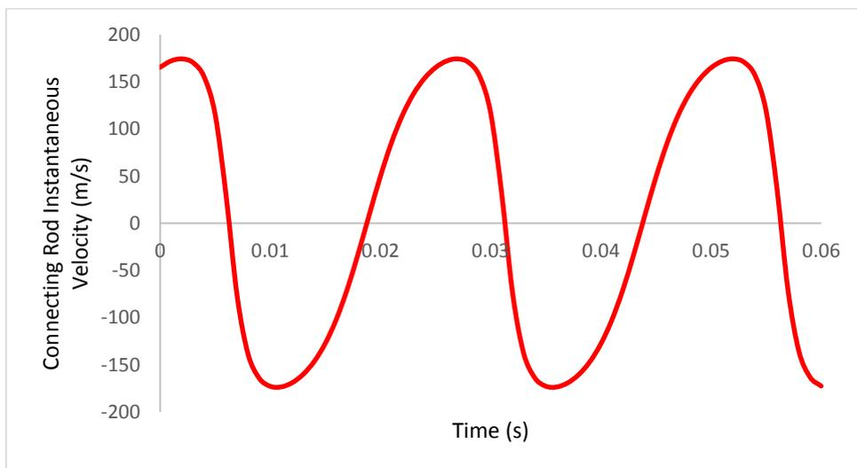
**Fig. 9:** Velocity-time graph of connecting rod
