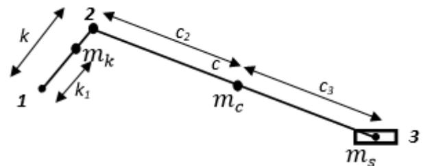
**Fig. 2:** Mass balance of offset slider-crank mechanism
