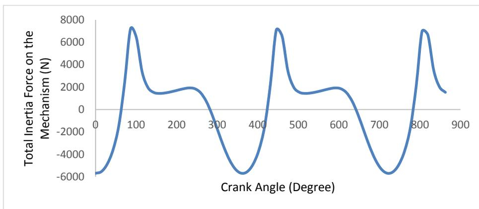
**Fig. 13:** Total inertia force on the mechanism
