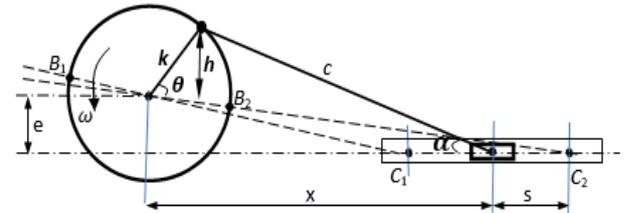
**Fig 1:** Offset slider-crank mechanism
