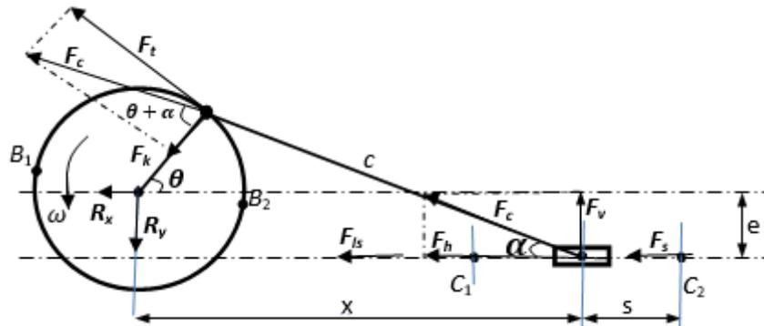
Fig. 3: Force analysis of offset slider-crank mechanism
