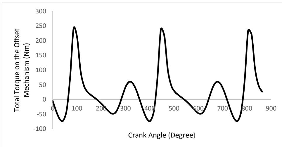
**Fig. 14:** Total torque on the mechanism
