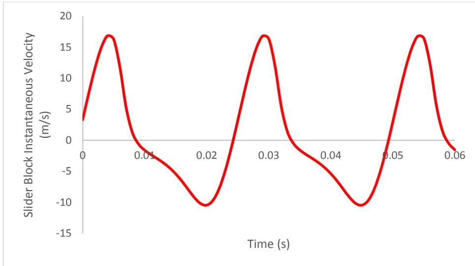
**Fig. 7:** Velocity-time graph of slider block
