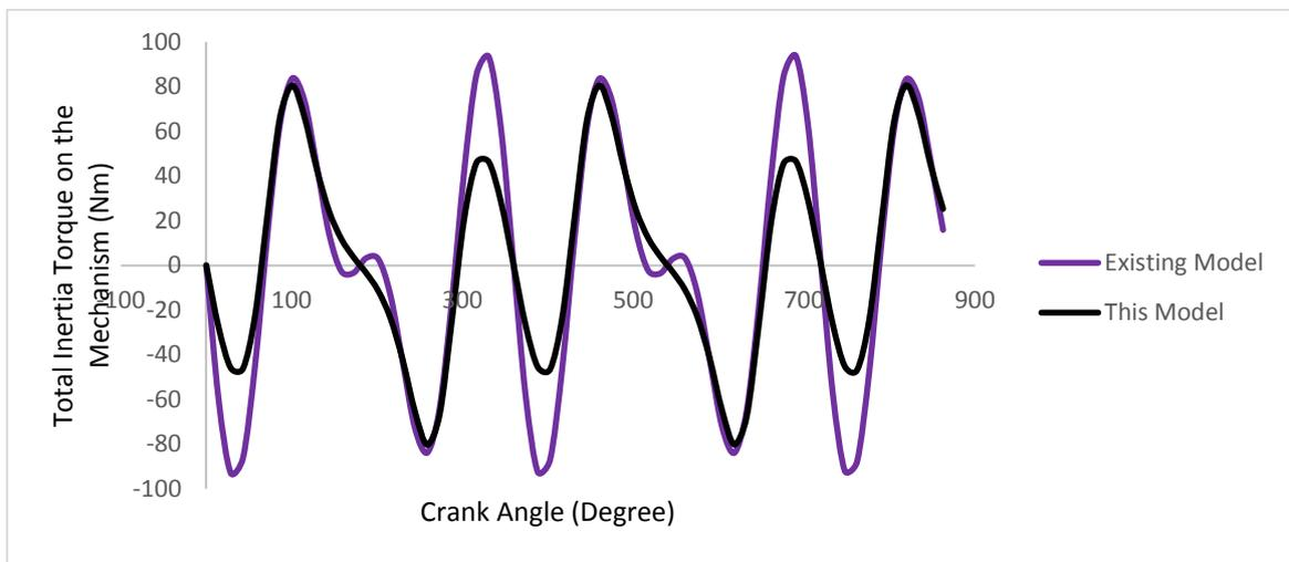
**Fig. 18:** Comparing torque with existing model at  $e = 0\text{mm}$
