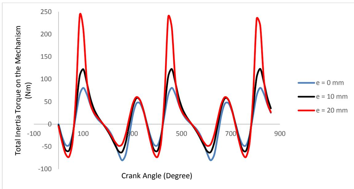
**Fig. 16:** Effect of offset distance on total torque
