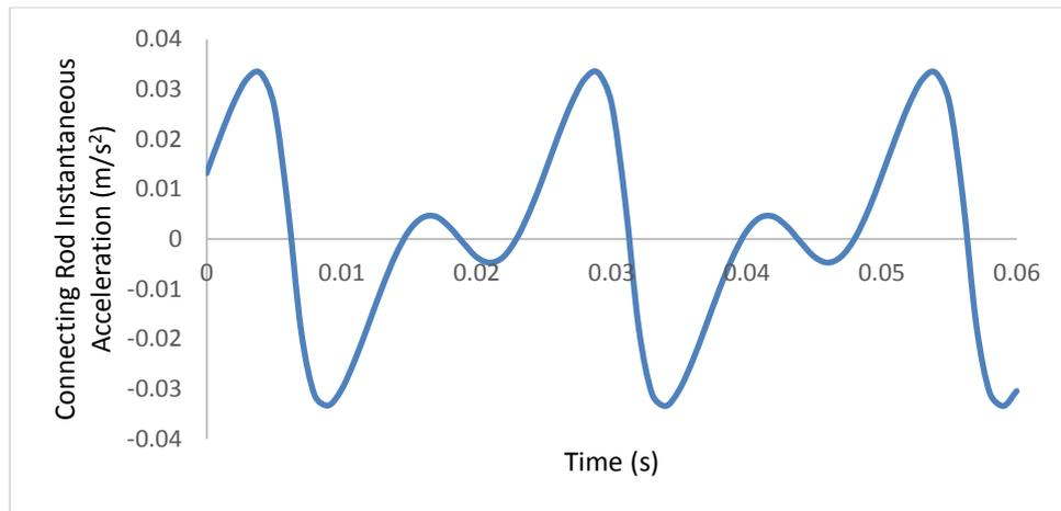
**Fig. 10:** Acceleration-time graph for connecting rod
