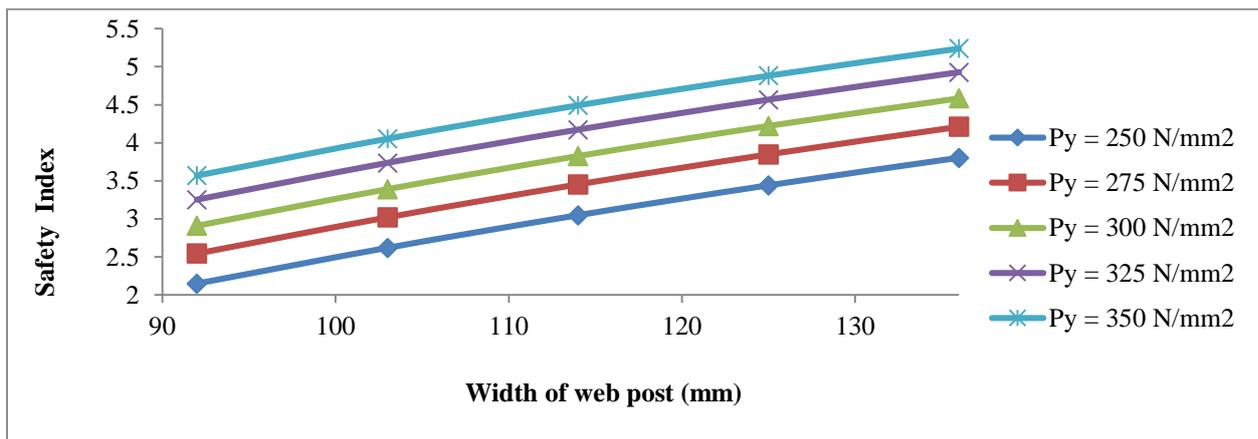
**Fig. 13:** Safety index against width of web post for varying bending strength (Horizontal shear criterion)
