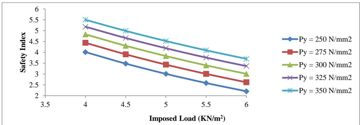
**Fig. 16:** Safety index against imposed load for varying bending strength (Shear criterion)
