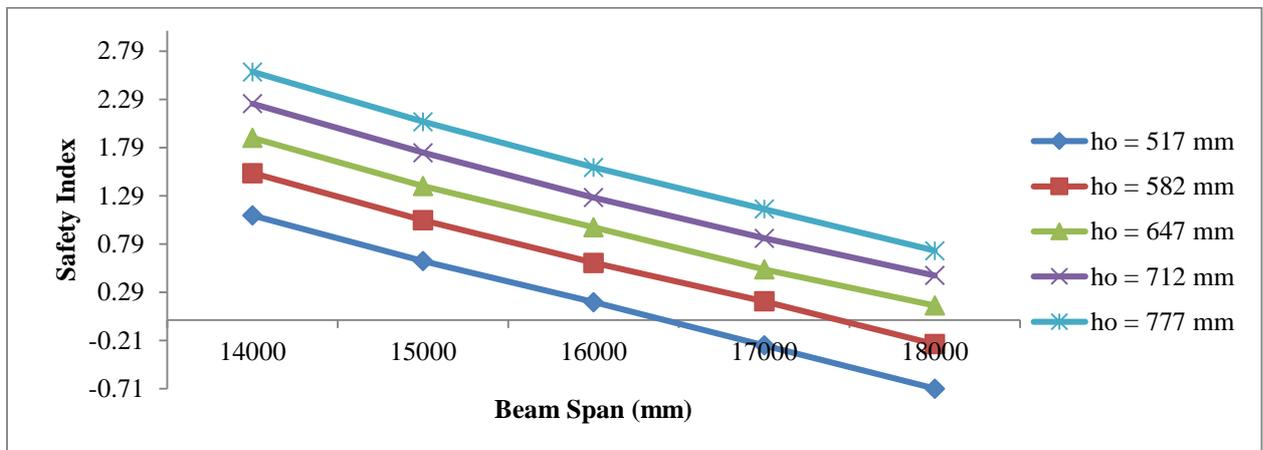
Fig. 6: Safety index against beam span for varying distance between the centroids of T-sections (Bending criterion)
