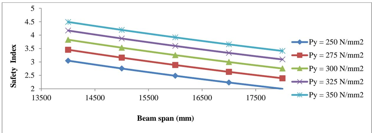
**Fig. 9:** Safety index against beam span for varying bending strength (Horizontal shear criterion)
