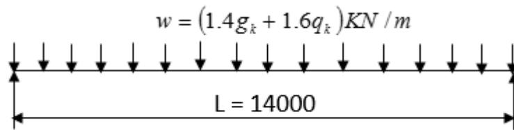
**Fig. 1a:** A castellated steel beam under uniform loading
