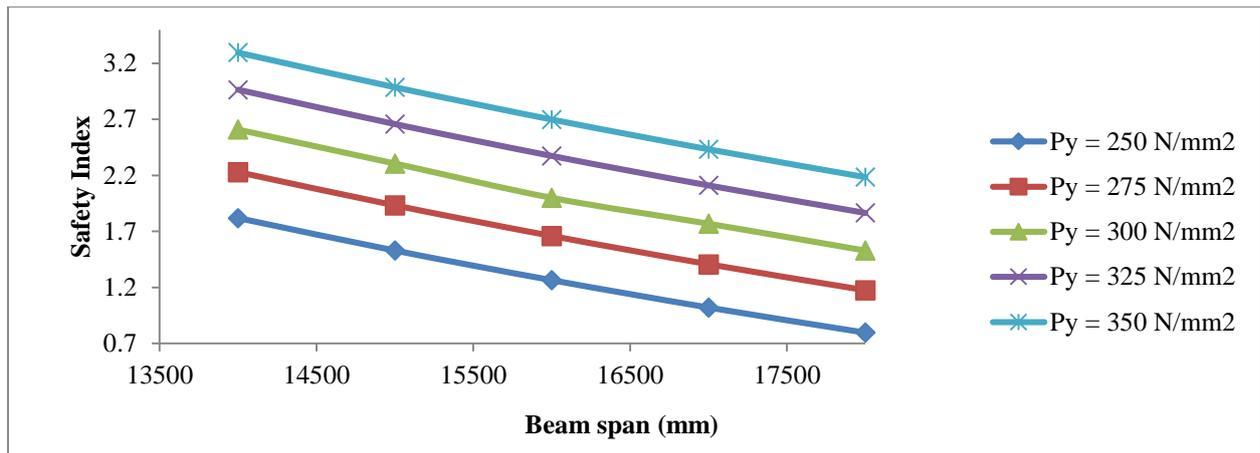
**Fig. 17:** Safety index against beam span for varying bending strength (Shear criterion)
