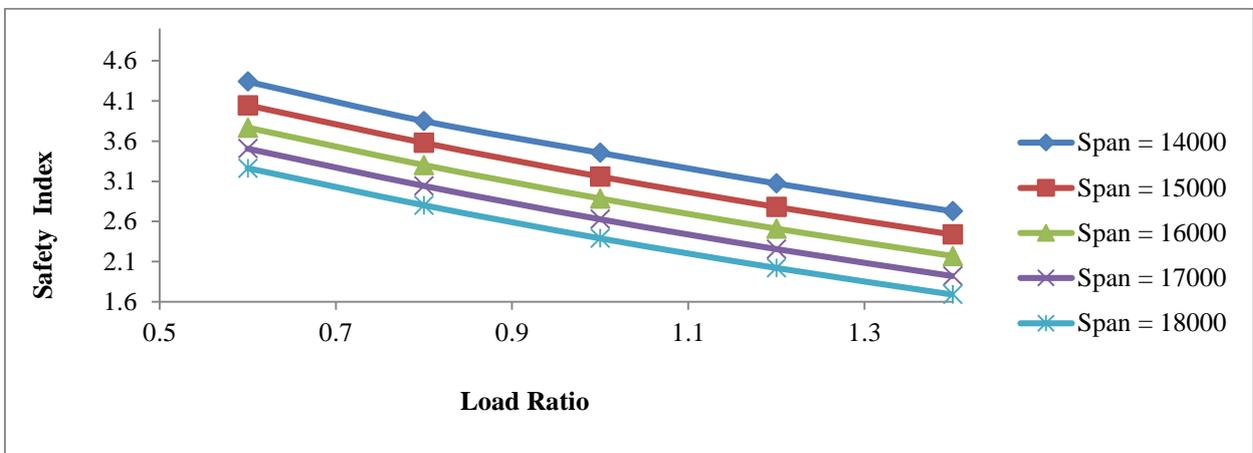
**Fig. 12:** Safety index against load ratio for varying beam span (Horizontal shear criterion)
