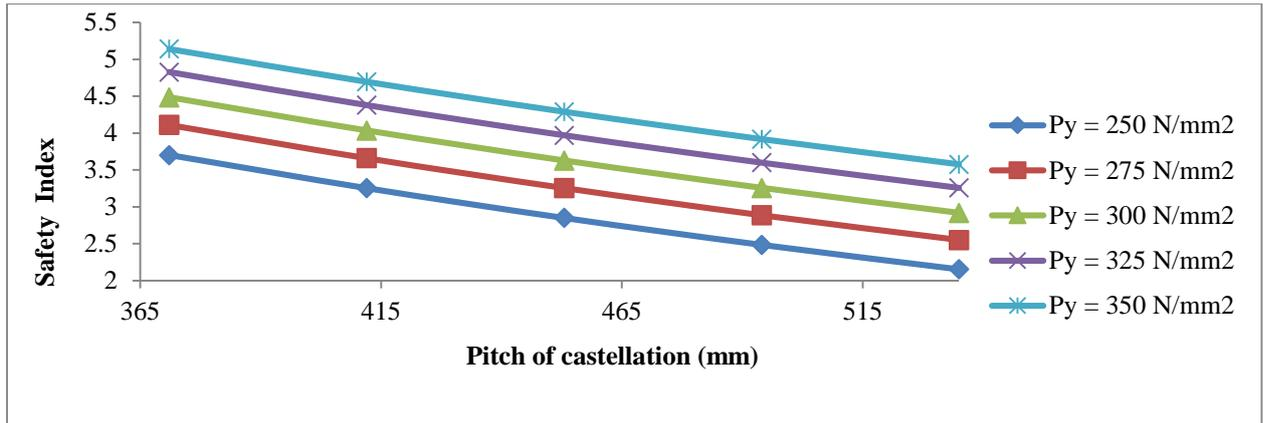
**Fig. 8:** Safety index against pitch of castellation for varying bending strength (Horizontal shear criterion)
