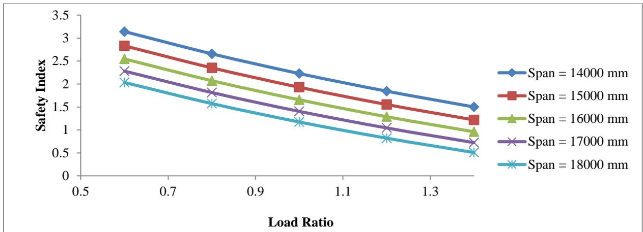
**Fig. 14:** Safety index against load ratio for varying beam span (Shear criterion)
