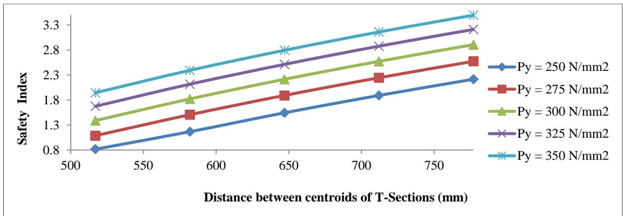
Fig. 7: Safety index against distance between centroids of T-sections for varying bending strength (Bending criterion)
