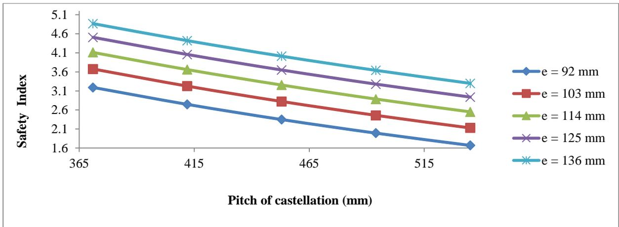
**Fig. 11:** Safety index against pitch of castellation for varying width of web post (Horizontal shear criterion)
