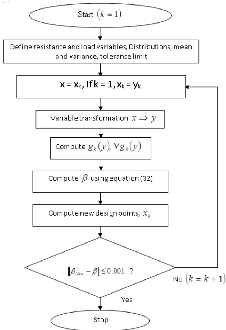
**Fig. 2:** Flowchart showing the optimization algorithm
