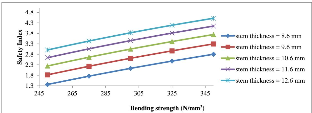
**Fig. 15:** Safety index against bending strength for varying thickness of stem of T-section (Shear criterion)
