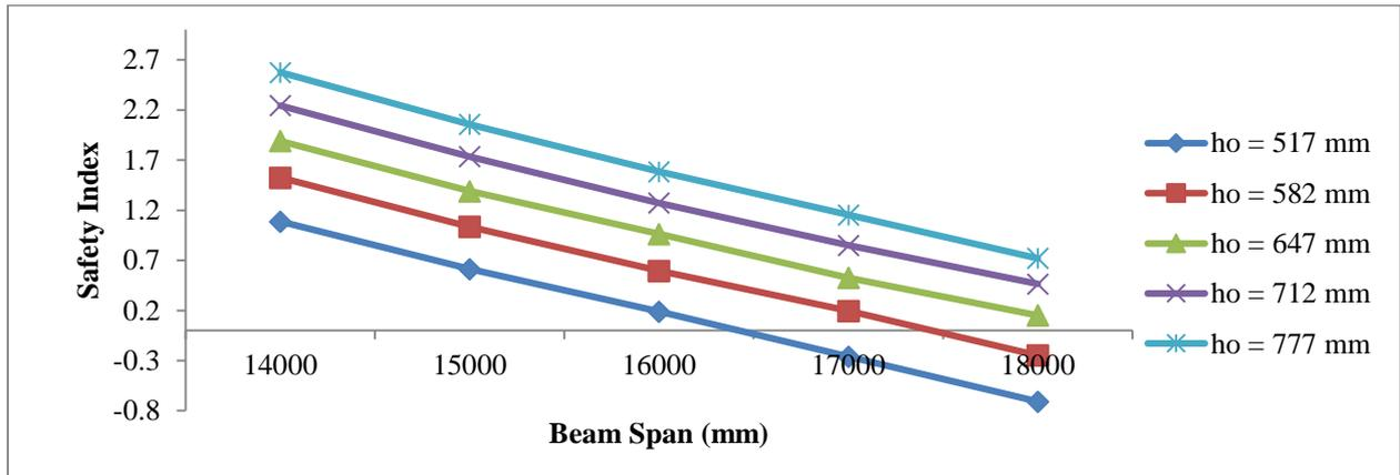
**Fig. 3:** Safety index against load ratio for varying beam span (Bending criterion)
