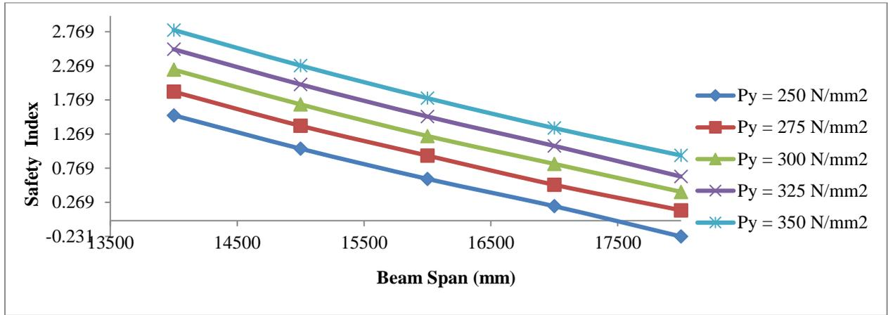
Fig. 5: Safety index against beam span for varying beam strength (Bending criterion)
