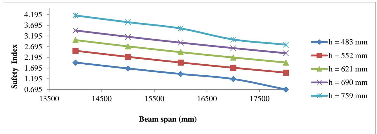
**Fig. 10:** Safety index against beam span for varying overall depth of beam (Horizontal shear criterion)
