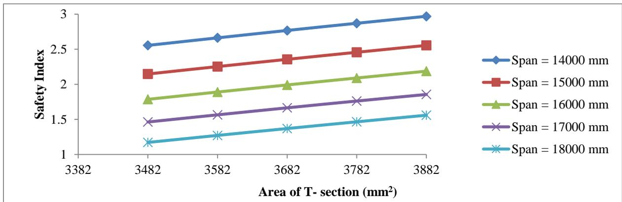
**Fig. 4:** Safety index against area of Tee-sections for varying beam span (Bending criterion)
