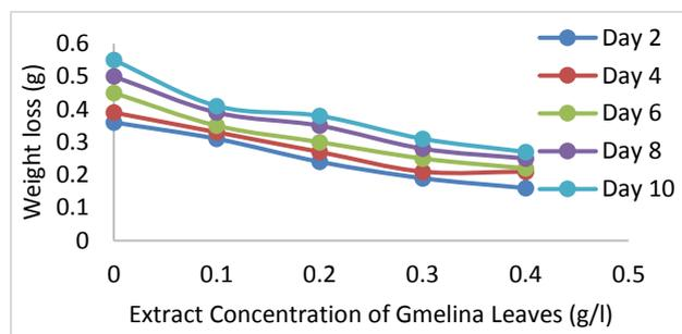
Fig. 2: Effect of Gmelina leaves extract concentration on weight loss of mild steel.
