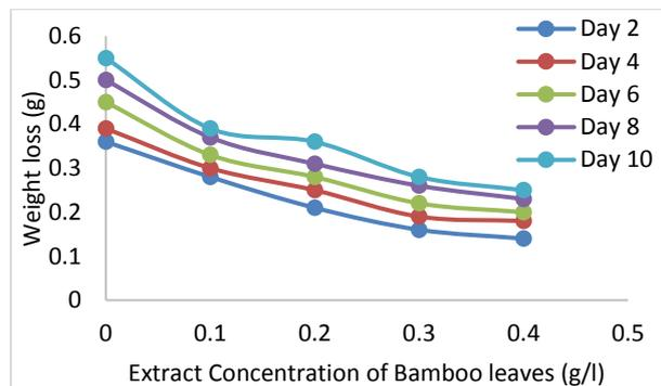
Fig. 1: Effect of Bamboo leaves extract concentration on weight loss of mild steel.
