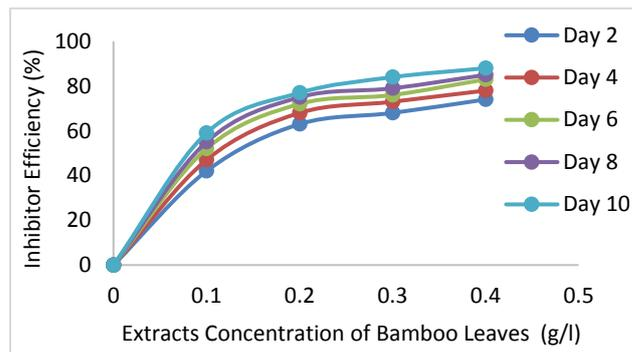
Fig. 3: Effect of Bamboo leaves extract concentration on inhibition efficiency.
