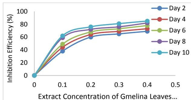
Fig. 4: Effect of Gmelina leaves extract concentration on inhibition efficiency.
